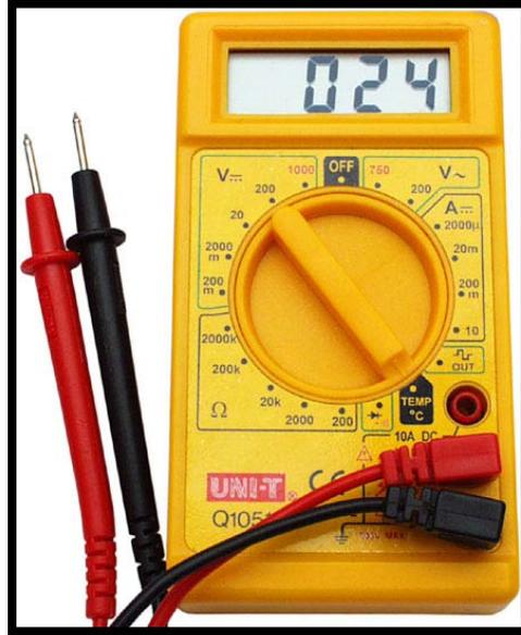
Digital multimeter is ok but we should note that we are using pulse DC in the SSG so when you are measuring the amps, it is highly recommended to use an Analogue Amp Meter, which goes up to 1amp or more. You will also need the meter to measure your input amps as well your battery voltages.
